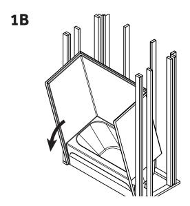
Tilt the fixture forward so that the front flanges rest on the floor.
