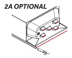
Optional: Instead of using the supplied mat, construction adhesive may be applied along the front threshold and along each rung of the support plate.
