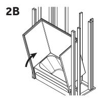
Return the fixture to the upright position aligning the fixture drain with the waste pipe location.
