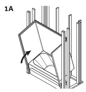
Place the fixture in the framed alcove and ensure that the floor is level and that the walls are plumb. The floor must be leveled prior to installation if it is greater than 1/8" from level.
