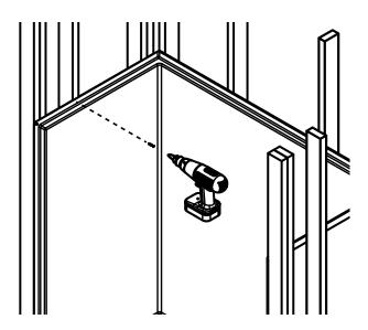
To secure the fixture to the stud walls, pre-drill holes every 16" along the vertical flanges and one hole per stud along the horizontal flanges. Nail or screw the fixture to the wall at each hole.
