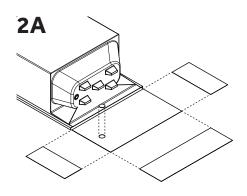
Cut or fold the edges of the supplied mat to match the fixture base dimensions as shown in the product submittal sheet. Cut a hole for the fixture drain.
